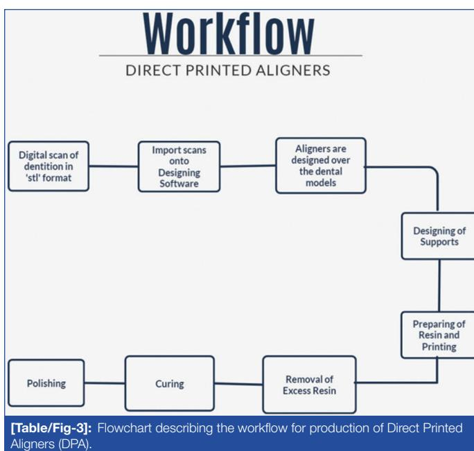
**[Table/Fig-3]:** Flowchart describing the workflow for production of Direct Printed Aligners (DPA).
